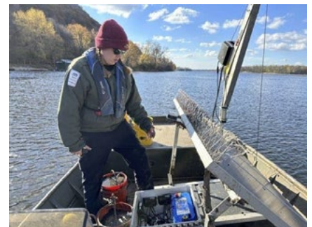
Minnesota DNR Invasive Carp Field Lead Kayla Stampfle inspects the components of a telemetry receiver that tracks tagged invasive carp in the Mississippi River near La Crosse. The solar-powered receiver can transmit real-time notifications of the movements of tagged invasive carp.
